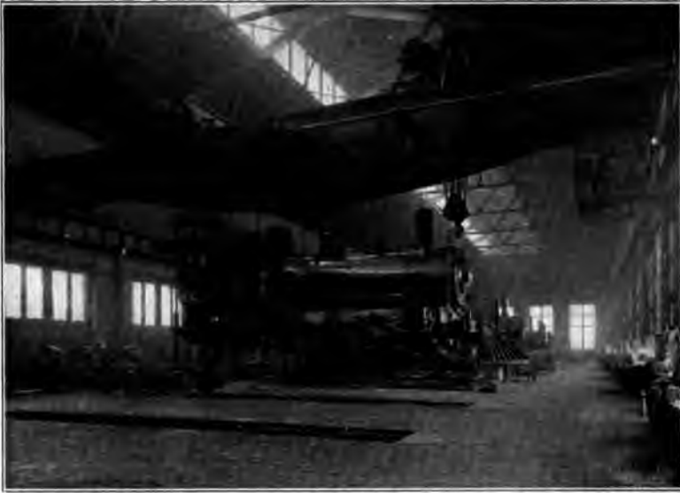
INSIDE THE WEST ALBANY SHOPS OF THE NEW YORK CENTRAL: PICKING UP A LOCOMOTIVE WITH THE TRAVELLING CRANE
